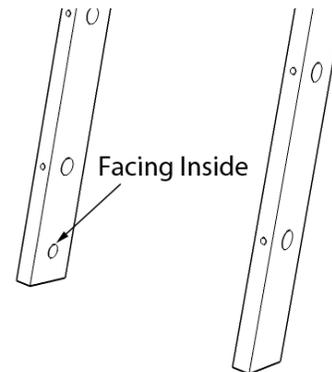
**Note:** Make sure the cam-lock screw holes at the bottom of the rack legs (2) are facing inside.
